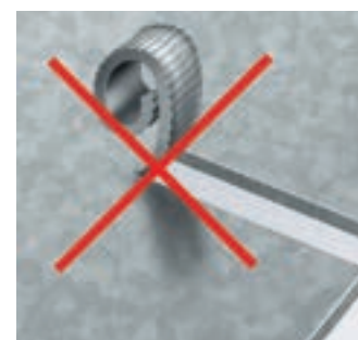
Notching without chip breaking
