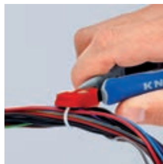
Remove the head of the cable tie using the Electronics Diagonal Cutter...
