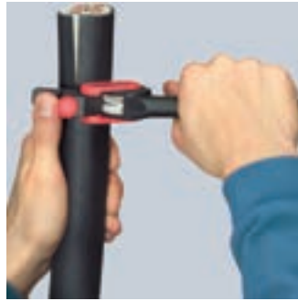
Turning the tool for circumferential cut
