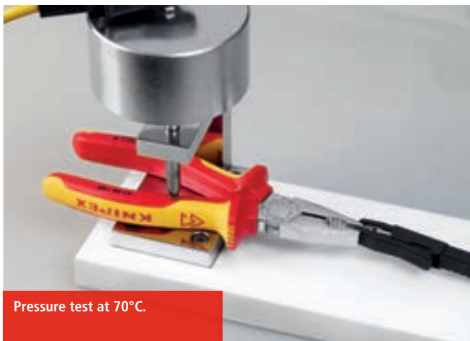
Testing the adhesion of the insulating coating at 500 N.
