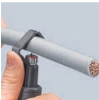
Setting the tool for circular cut
