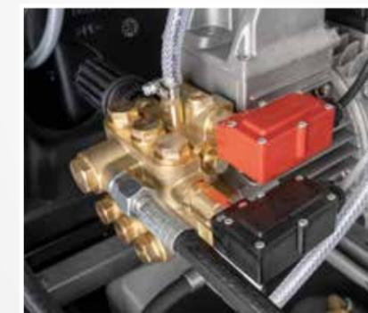
**TOTAL-STOP SYSTEM WITH DELAYED MOTOR SHUTDOWN**
